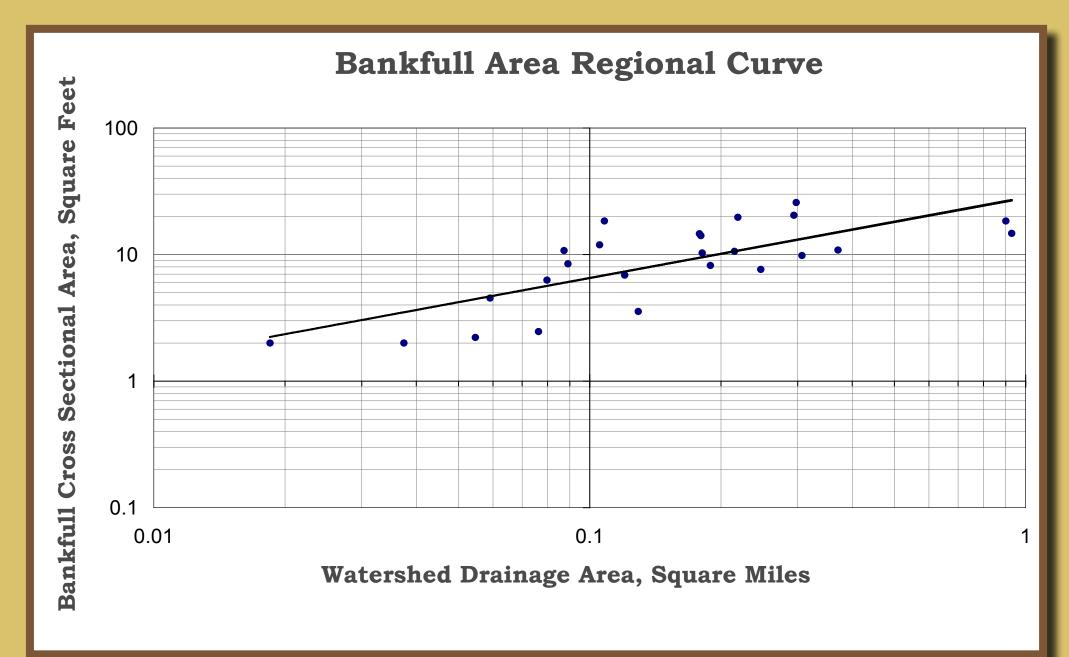
FIGURE 2. Typical site-specific "regional" curve relating bankfull cross-sectional area and drainage area
