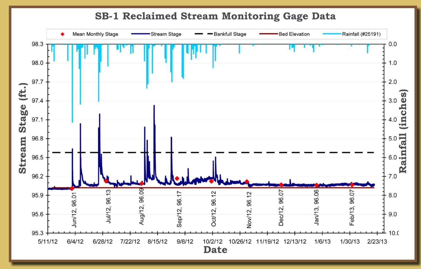
FIGURE 2. Stream stage hydrograph and rainfall data
