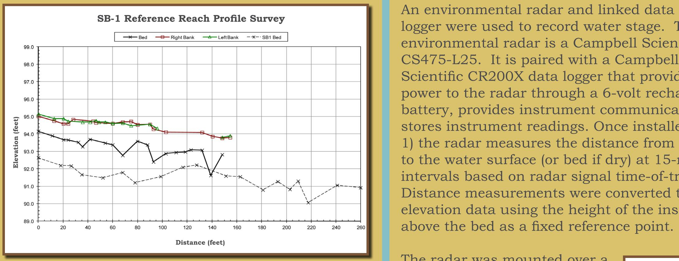
FIGURE 1. Bed profile survey of the restored stream channel compared to the reference stream profile
